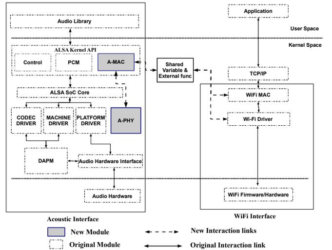
Fig. 7: Acoustic-WiFi architecture implementation in Smart devices
